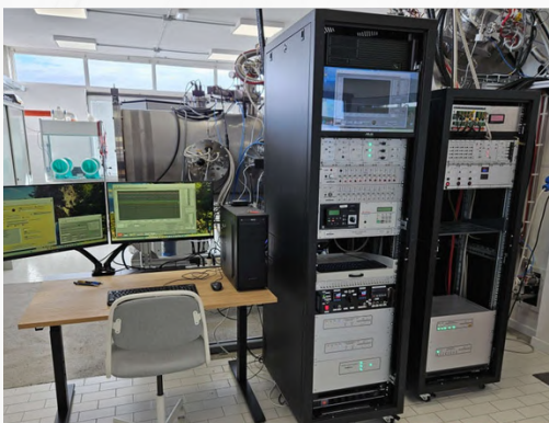
Vacuum Test Facility, auxiliary chamber and control desk
