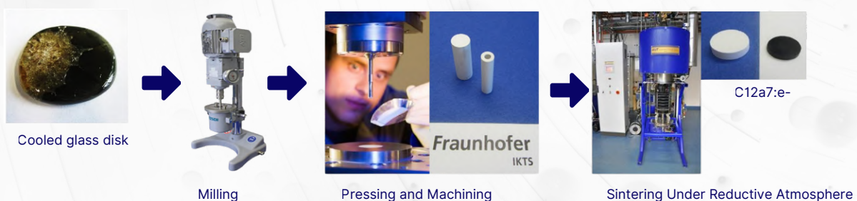
Picture 09 Processing steps for preparation of electron emitting C12A7 ceramic
