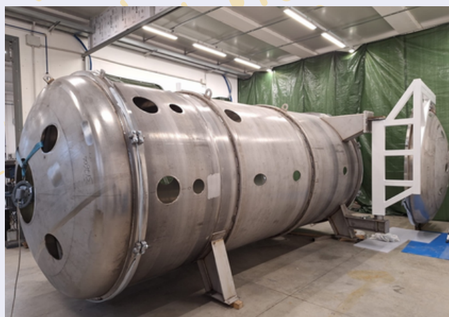
Figure 6. The main vacuum chamber of the new test facility
