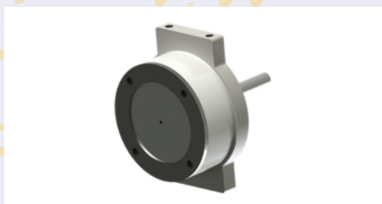
Figure 2. Render of the planar iodine cathode, designed to use C12A7 emitter disks manufactured by Fraunhofer IKTS.
